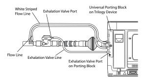
**Note**: When using an active exhalation device with proximal flow, ensure that any additional proximal ports are capped.
